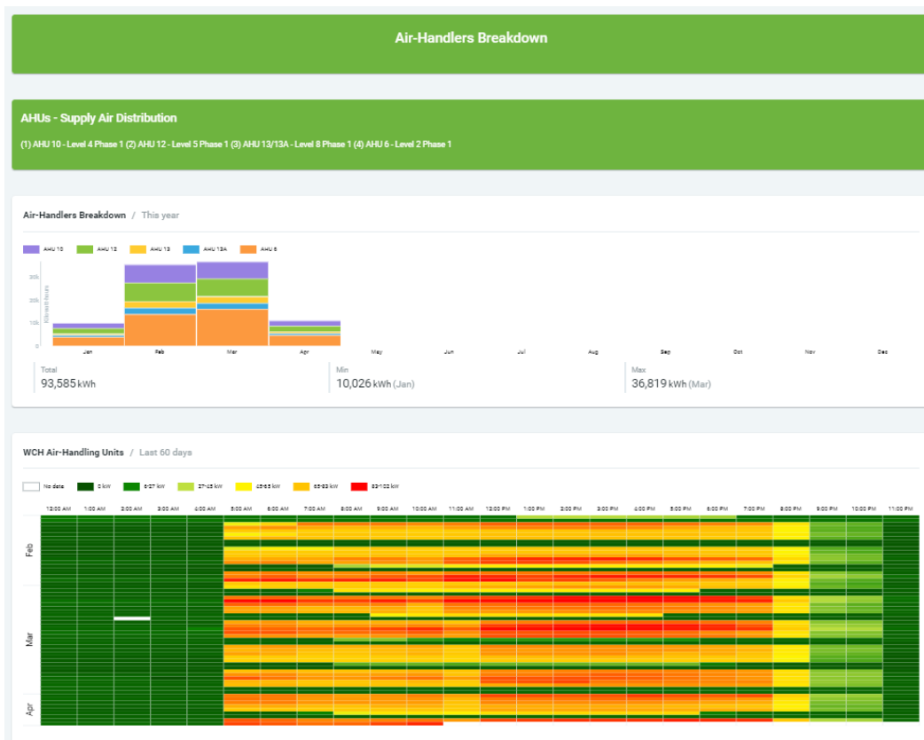
Figure 7: WCH AHU Operational Dashboard - Atrius
