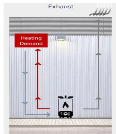
Figure 7: Conventional Heating System
